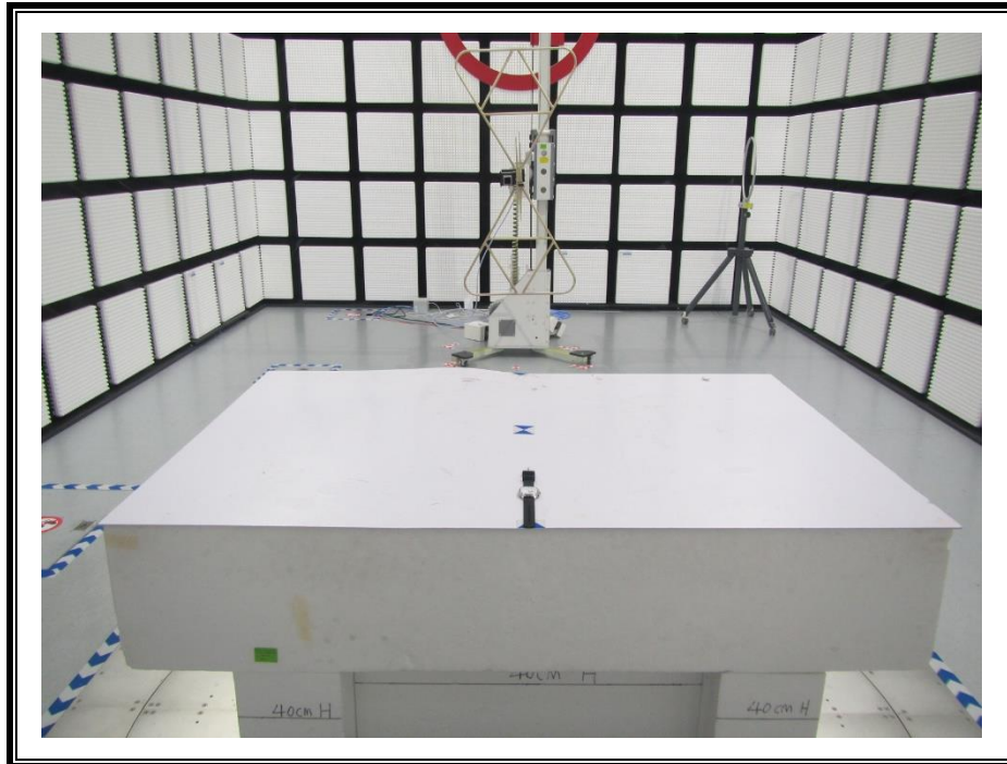
RADIATED RF MEASUREMENT SETUP (Below 30MHz)
