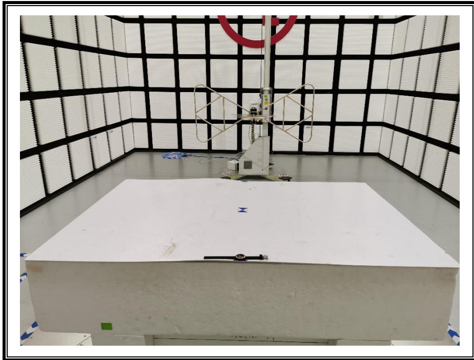
RADIATED RF MEASUREMENT SETUP (Below 30MHz)
