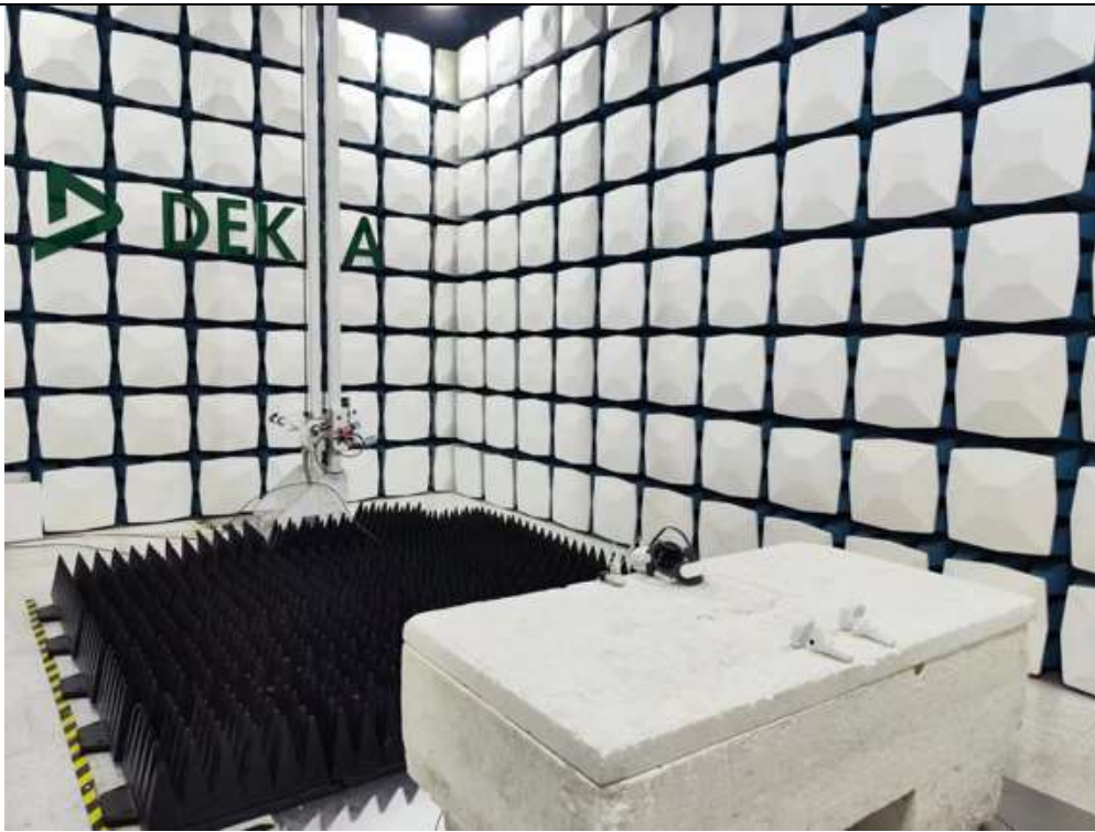
Description: Rear View of Radiated Disturbance Test Setup (1-18 GHz)
