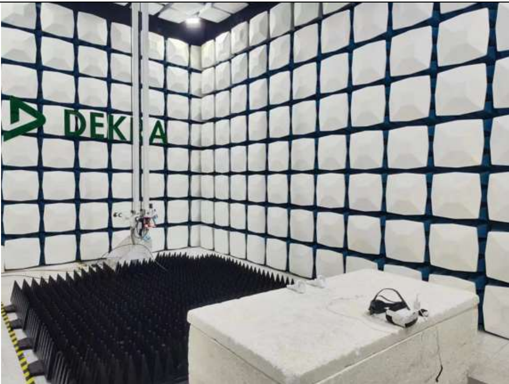
Description: Rear View of Radiated Disturbance Test Setup (1-18 GHz)
