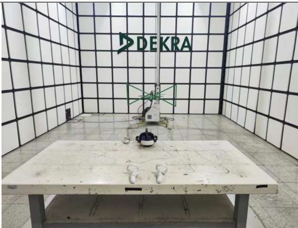
Description: Rear View of Radiated Disturbance Test Setup (Below 1 GHz)
