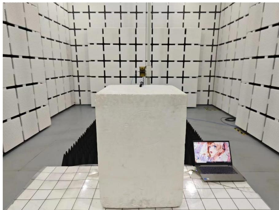
**Conducted Emission Test Setup Photo**
