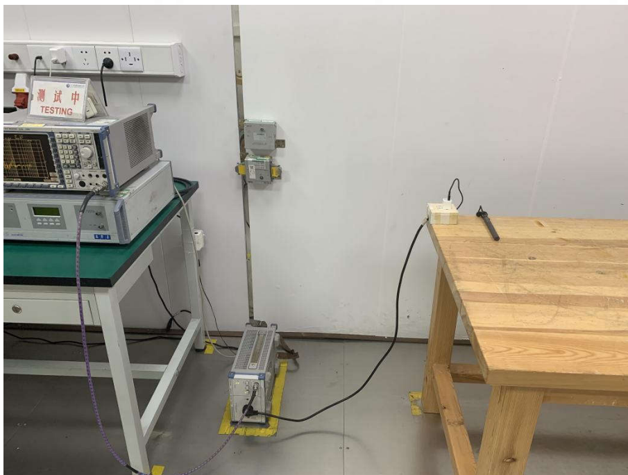
Conducted Emissions Test Setup
