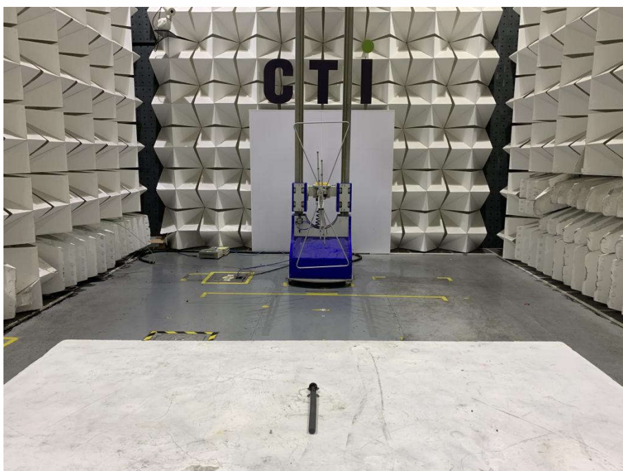
Radiated spurious emission Test Setup-1(Below 1GHz)
