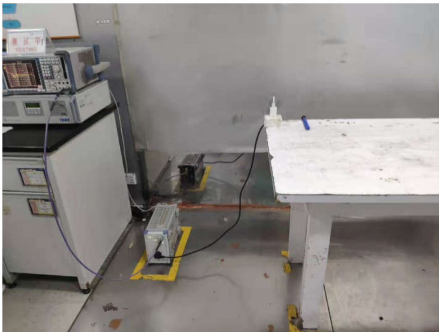
Conducted Emissions Test Setup
