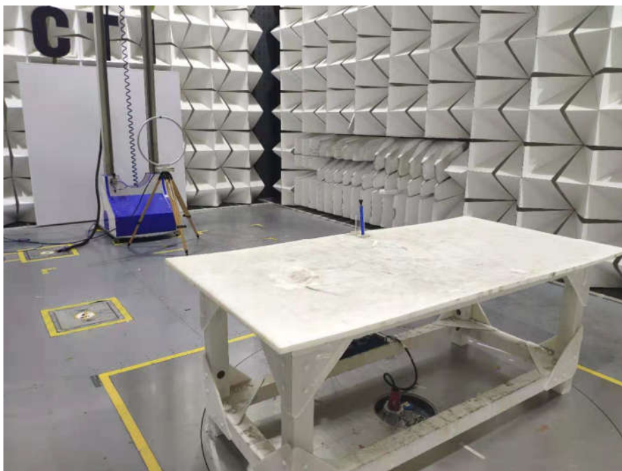
Radiated spurious emission Test Setup-1(Below 30MHz)
