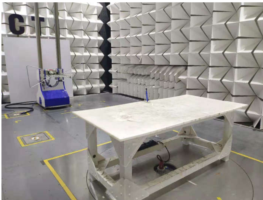
Radiated spurious emission Test Setup-1(Below 1GHz)
