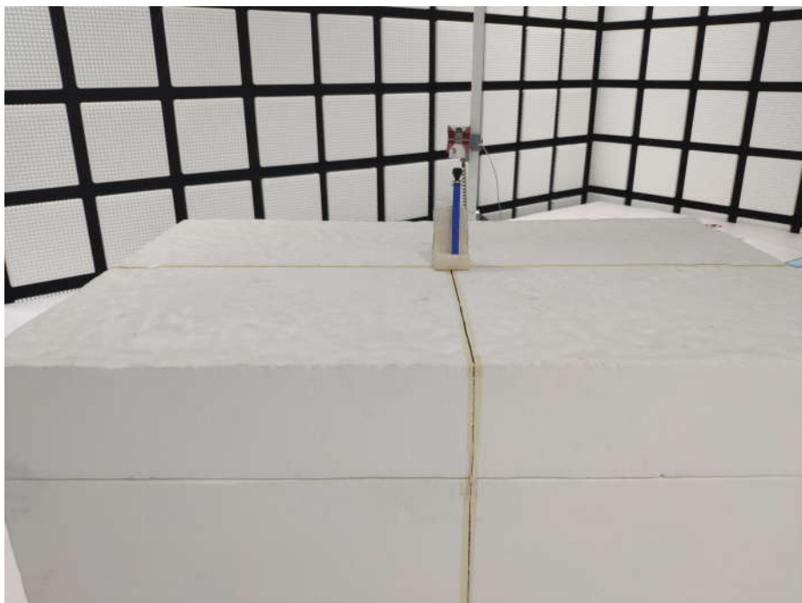
Radiated spurious emission Test Setup-2(Above 1GHz)
