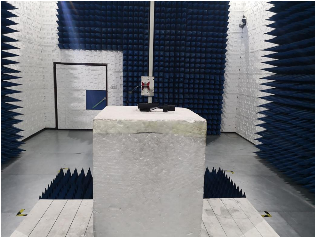
FCC RADIATED EMISSION TEST SETUP ABOVE 1GHZ
