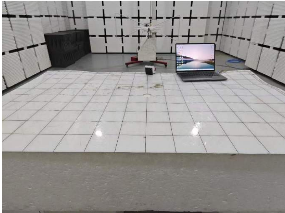
Set-up for Radiated Spurious Emission, Above 1GHz
