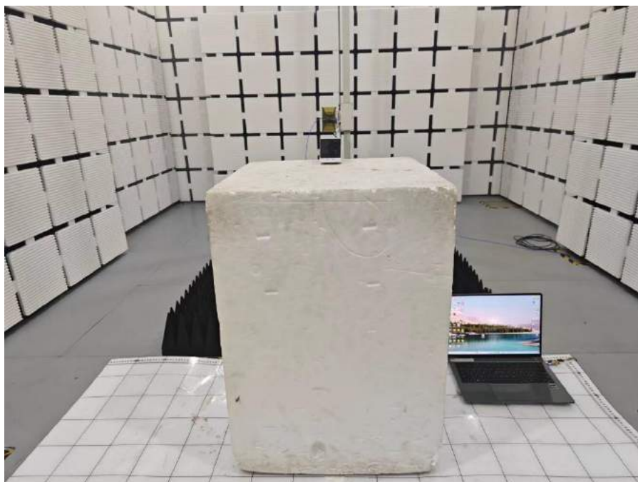
Set-up for Radiated Spurious Emission, Above 1GHz
