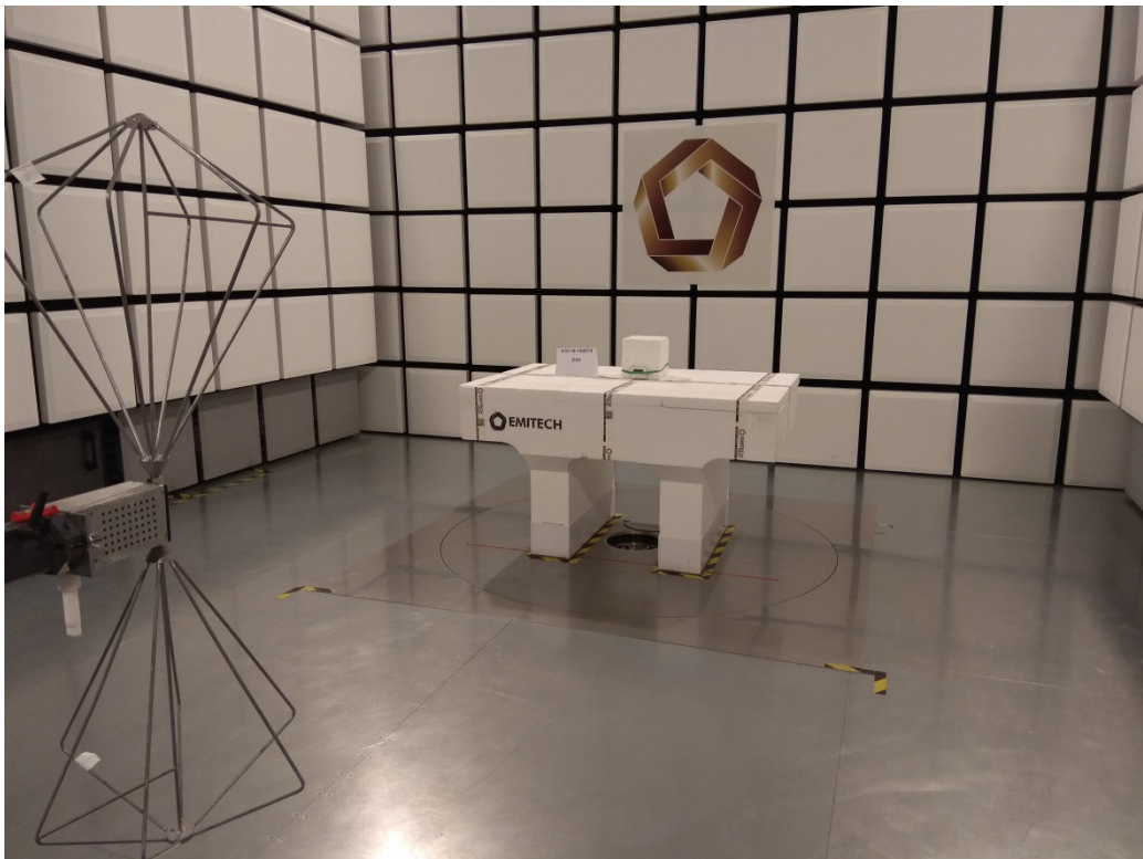
TEST SETUP PHOTO(S) - SPURIOUS – 30MHZ TO 200 MHZ
