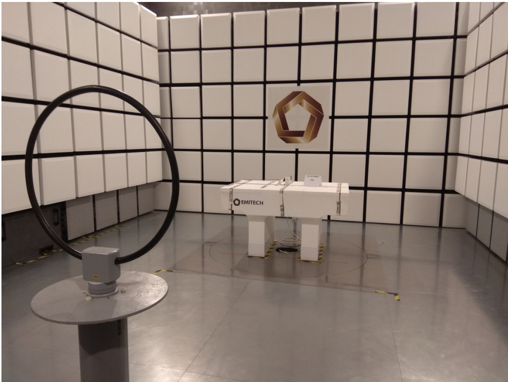
TEST SETUP PHOTO(S) – SPURIOUS – 9KHZ TO 30 MHZ
