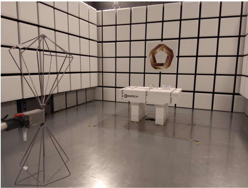
TEST SETUP PHOTO(S) - SPURIOUS – 30MHZ TO 200 MHZ
