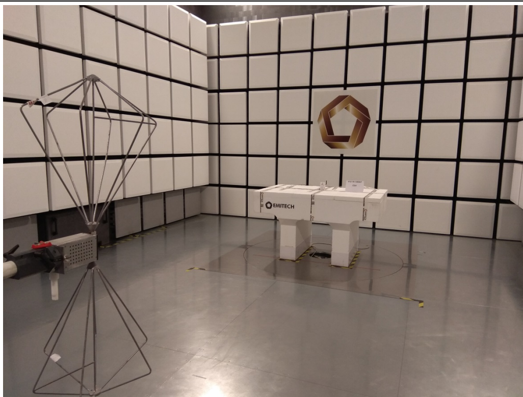
TEST SETUP PHOTO(S) - SPURIOUS – 30MHZ TO 200 MHZ
