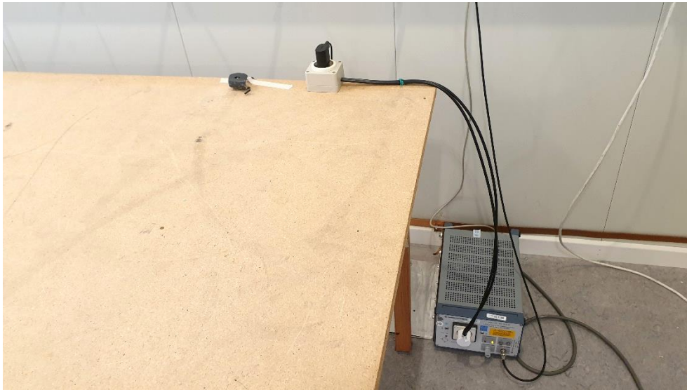
Photo 13. AC Conducted emission test set up. Powered by AC/DC adaptor.
