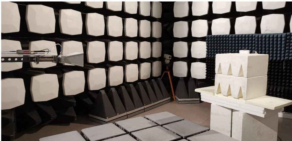
Photo 8 - Radiated emission test setup for 1 – 14 GHz.
