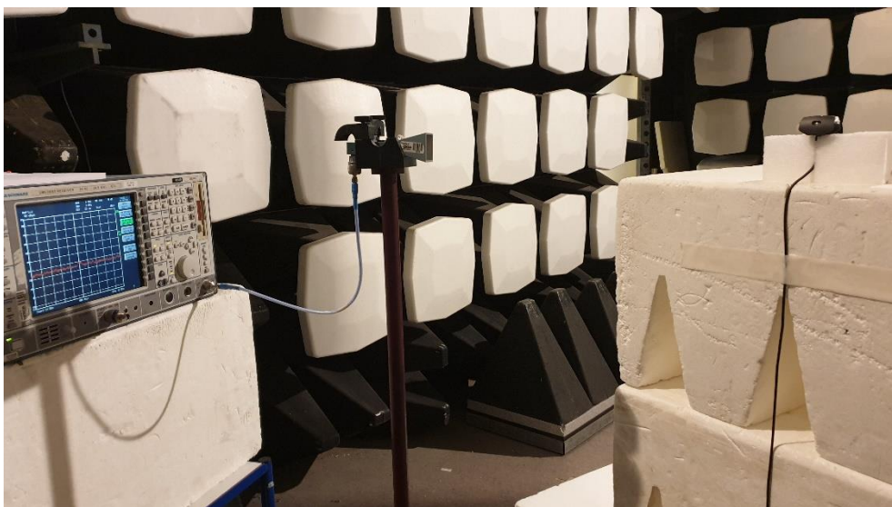
Photo 9. Radiated emission test setup for 14 – 25 GHz.
