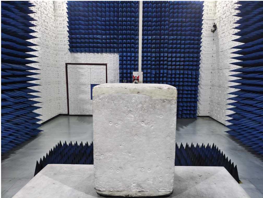
RADIATED EMISSION TEST SETUP ABOVE 1GHz
