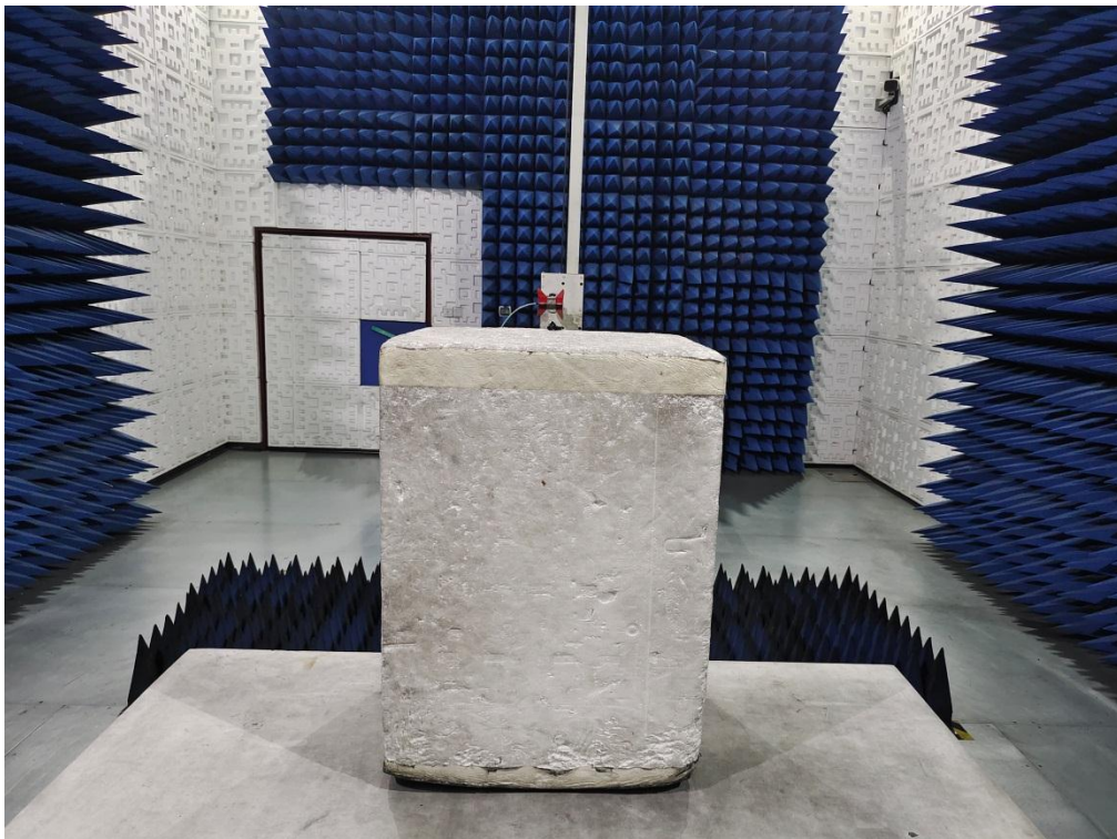
RADIATED EMISSION TEST SETUP ABOVE 1GHz
