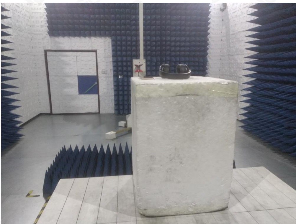
RADIATED EMISSION TEST SETUP ABOVE 1GHZ
