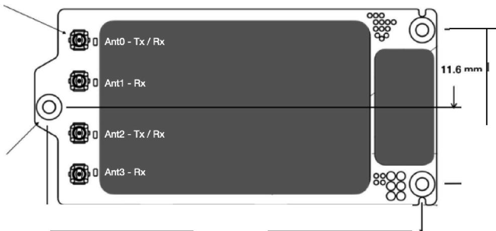
On the antenna cable, the mating connector is an I-PEX 20278-112R series connector. Antenna types and gains must follow the FCC / IC regulatory filings submitted by Skydio.
