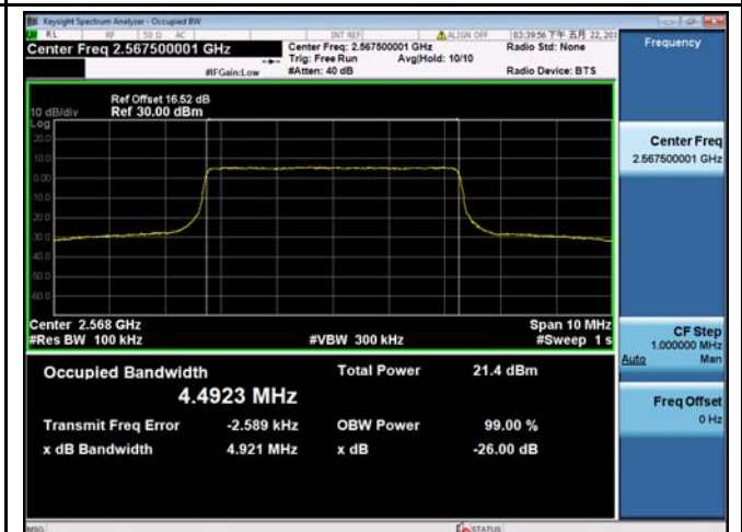
LTE band 7 - Middle CH 16QAM-5
