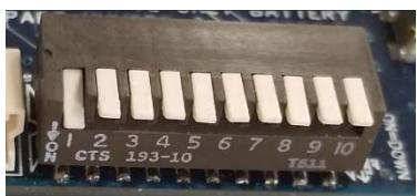
**Dip Switches Student Unit:** This shows a Phone Locker Dip Switch and is not part of the Teacher Unit. To Pair a Phone Locker with the example Teacher unit above, we would use the same code of 1000000000. Switching switch 1 down towards the ON label will activate it "on" which equals 1. The remaining switch position 2-10 for our example are in the UP position which is off or 0. Our example teacher unit and our phone locker are now paired. A teacher unit may control up to 100 phone lockers.
