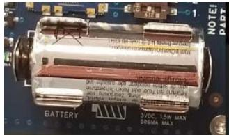
**Battery:** This battery is **not** rechargeable. Use only a new cr123a non rechargeable lithium battery for replacement. Recycle battery according to local rules and regulations. Battery life will depend on frequency of use.
