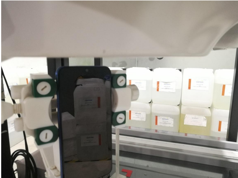
Top Edge(separation distance is 10mm)
