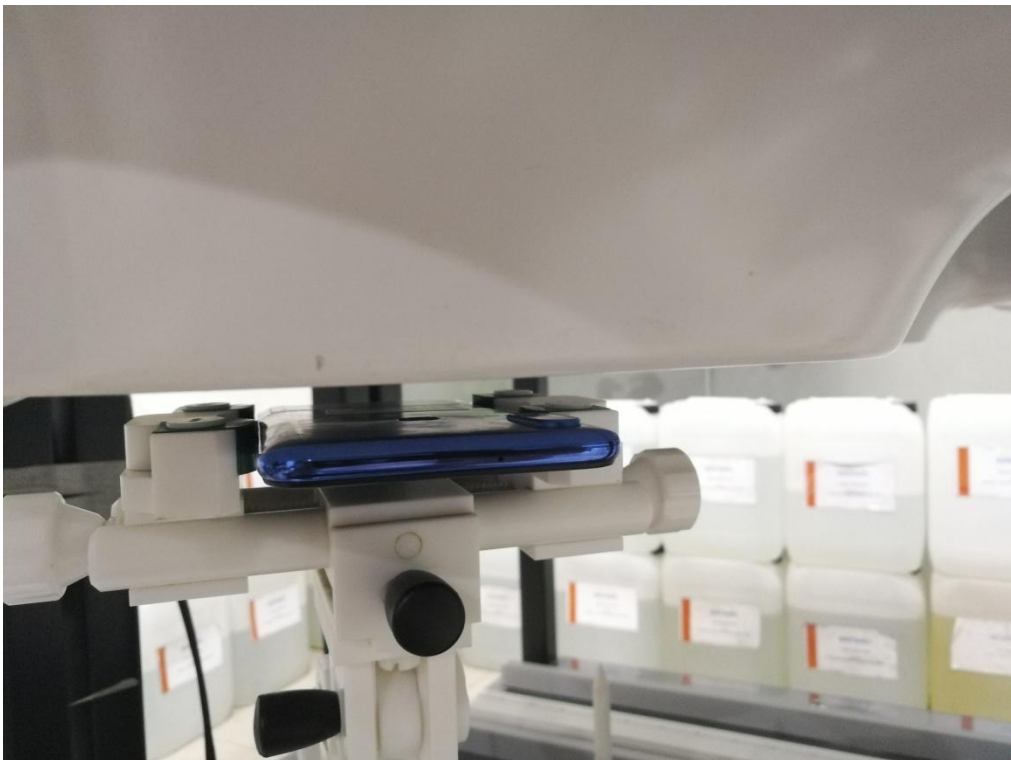
Back side(separation distance is 10mm)
