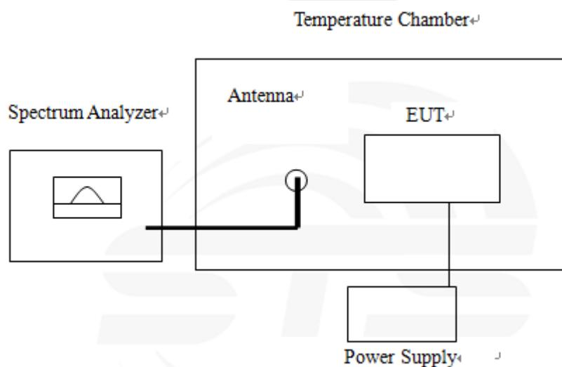
The EUT which is powered by the Battery, is coupled to the Spectrum Analyzer; the RF load attached to the EUT antenna terminal is 50Ohm; the path loss as the factor is calibrated to correct the reading.
