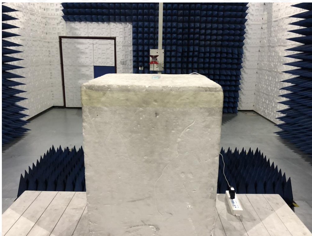
FCC RADIATED EMISSION TEST SETUP ABOVE 1GHZ
