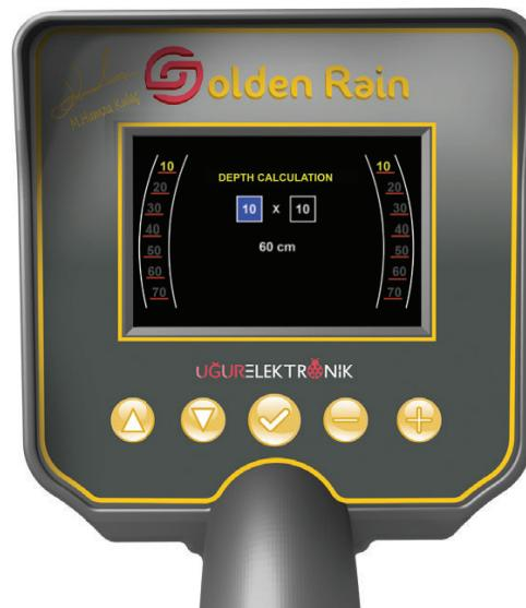
To calculate the length and width of the signal, measure signal from the first place to the end of it (width) and repeat the same for the other part (length). Upon determination of the sizes, press button for 2 seconds and open depth calculation section. Choose the nearest dimensions to those you have estimated. The depth will be calculated automatically and depending on the depth, there is 10 and 50 cm margin or error.
