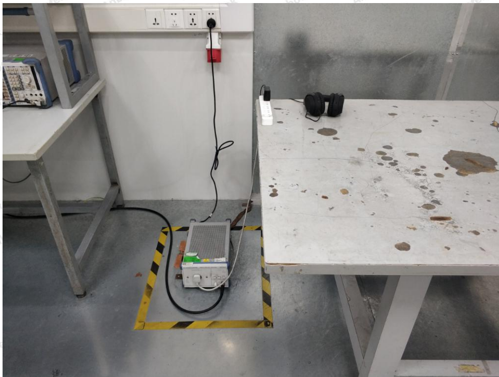
Photo of Conducted Emission Measurement
