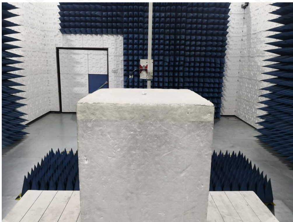
RADIATED EMISSION TEST SETUP ABOVE 1GHZ
