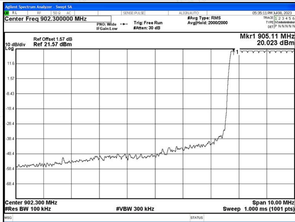
Band Edge(Hopping) NVNT 902.3MHz Ant1 Hopping Emission
