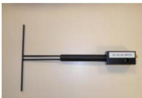
Figure 1 – Satimo COMOSAR Validation Dipole
