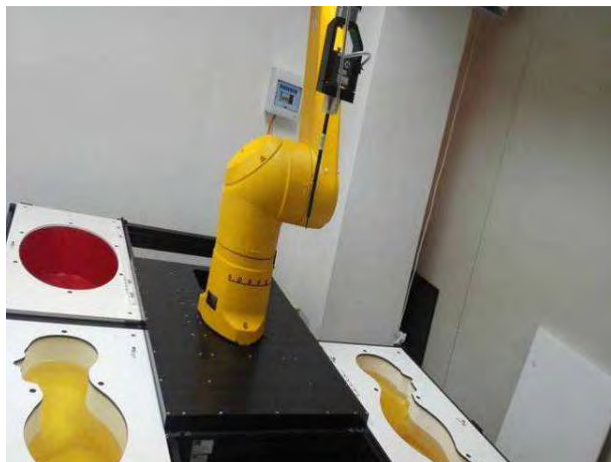
Specific Absorption Rate Test Layout
