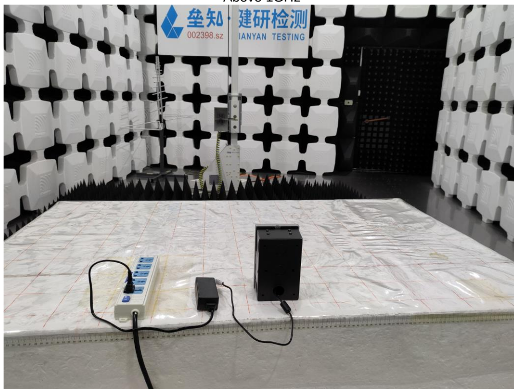
Radiated Emission(DC power supply) Above 1GHz
