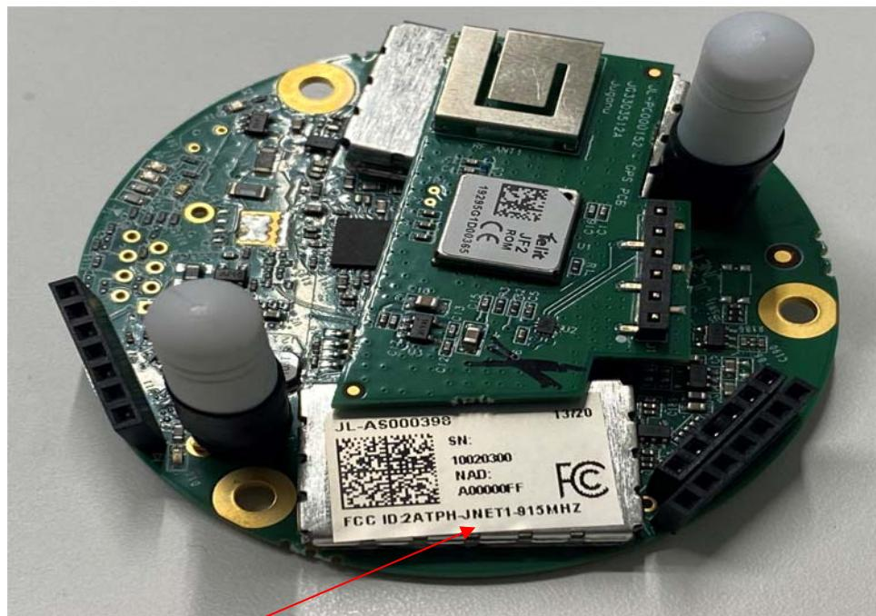
Label with FCC ID:2ATPH-JNET1-915MHZ is placed here.
