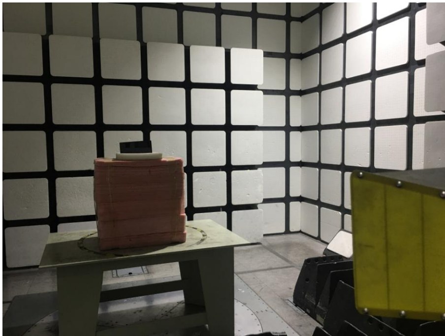
Radiated Emissions View (Above 1 GHz)
