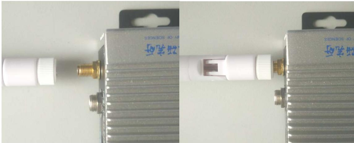
The connecting method of antenna extension cables: Take an antenna extension cable out of the packaging bag, align it with the position of an antenna joint, and rotate the nut clockwise until tight. The schematic diagram of connecting an antenna extension cable is given as follows:
