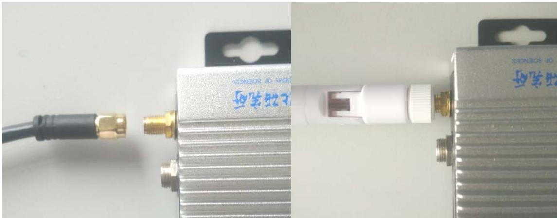
Note: Either antennas or antenna extension cables can be installed on a WIA-FA wireless communication device.
