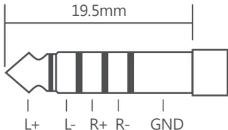
For 4.4mm Balanced to dual XLR connections, the balanced output should be wired as follows:
