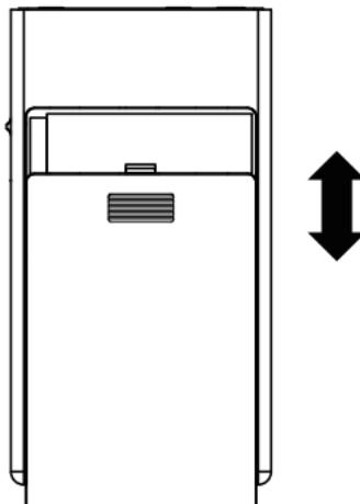
Open the back cover to change the amplifier card. In order to customise for different headphones, earphones and customers, HIFIMAN provides a variety of amp cards to choose from. Please see the following diagram for the steps to replace the amplifier card:
