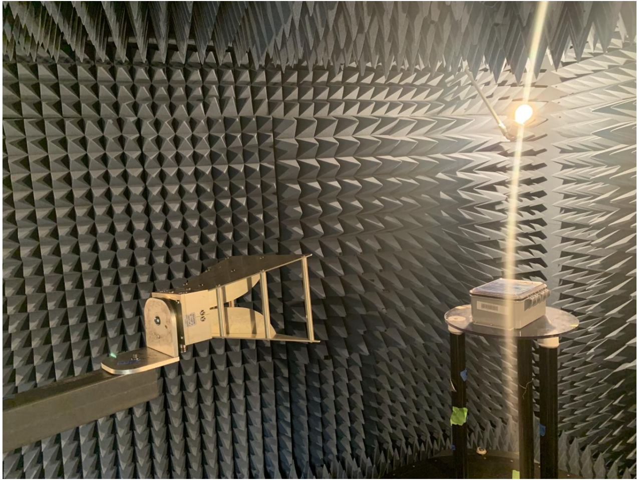
Photograph 2. Radiated Emission Test Setup - 1 GHz – 18 GHz
