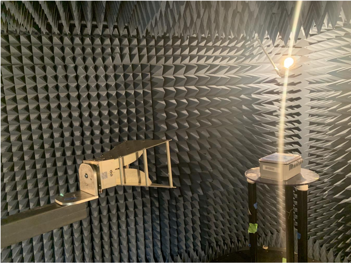
Photograph 7. Radiated Emissions Test Setup
