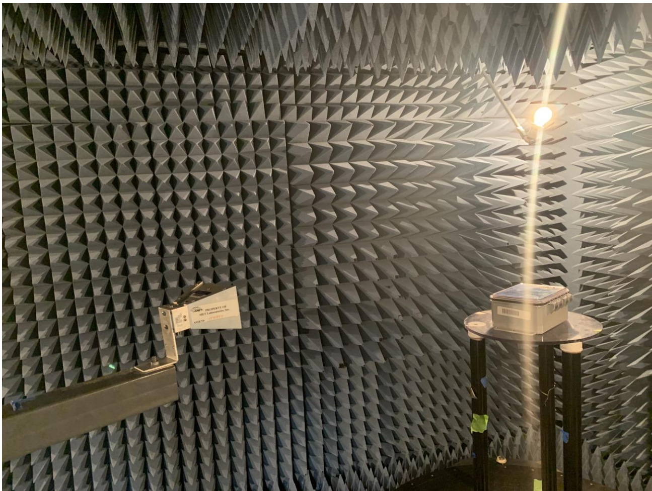
Photograph 6. Radiated Emission Test Setup - 18 GHz – 40 GHz
