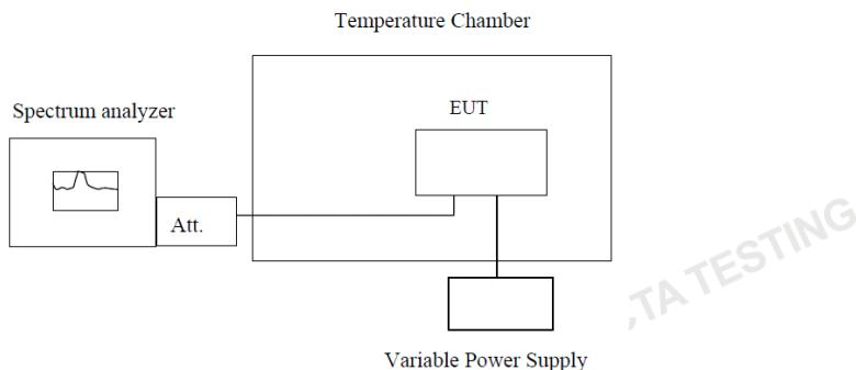
**Note :** Measurement setup for testing on Antenna connector
