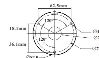
3. Route and connect the power cable and then secure the camera to the wall with screws as shown below.
