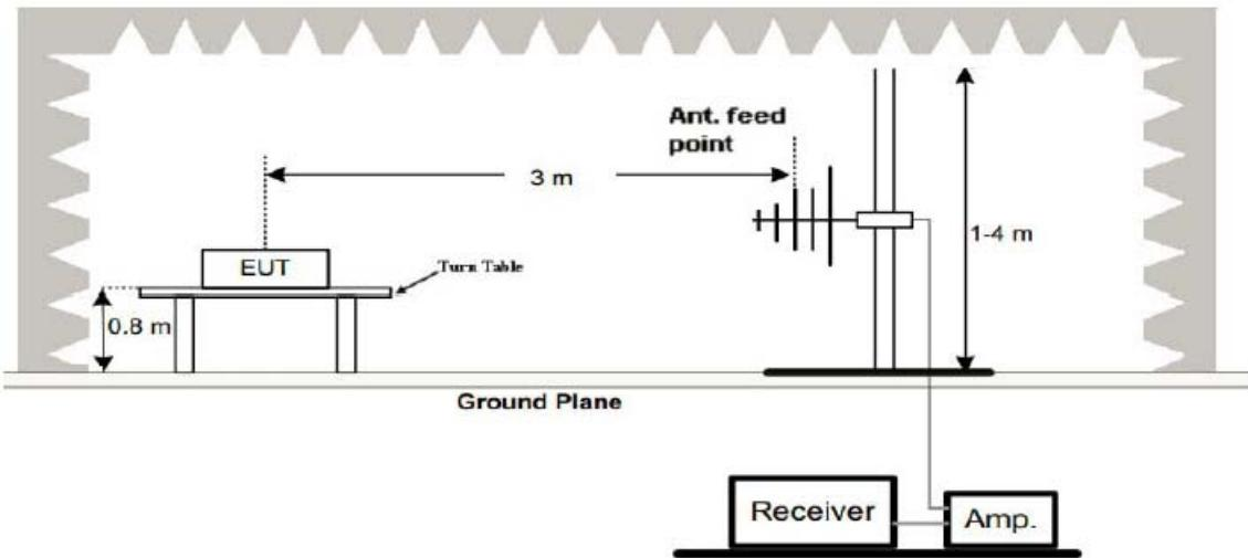
(3) Radiated Emission Test-Up Frequency Above 1GHz
