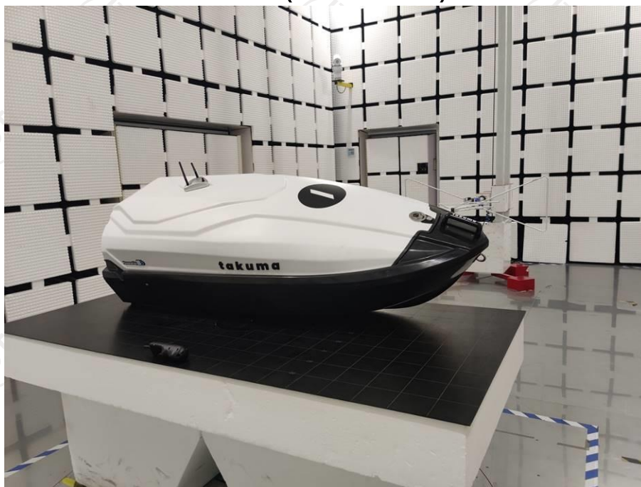
Radiated emission (30 MHz to 1 GHz) Test View
