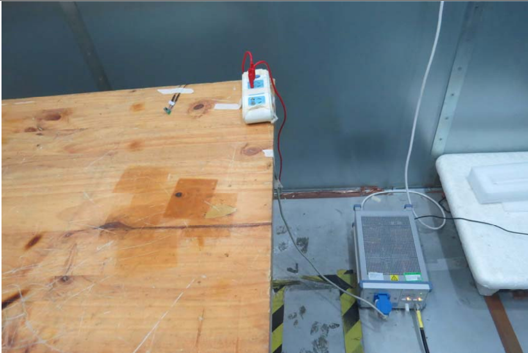
Picture 3 Conducted Emission Test Setup
