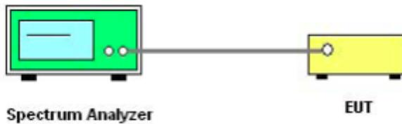
The EUT which is powered by the Battery, is connected to the Spectrum Analyzer; the RF load attached to the EUT antenna terminal is 50Ohm; the path loss as the factor is calibrated to correct the reading.
