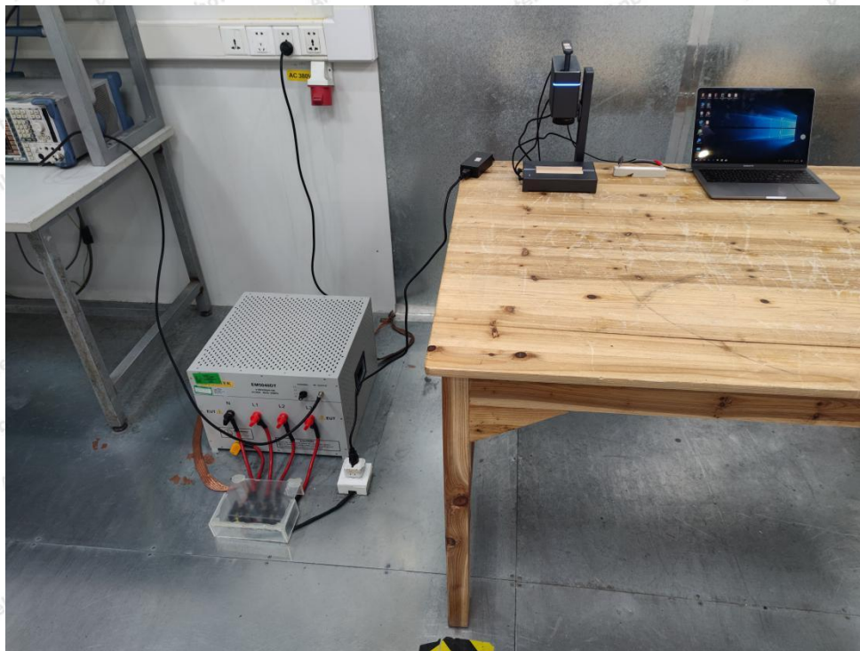
Photo of Conducted Emission Measurement
