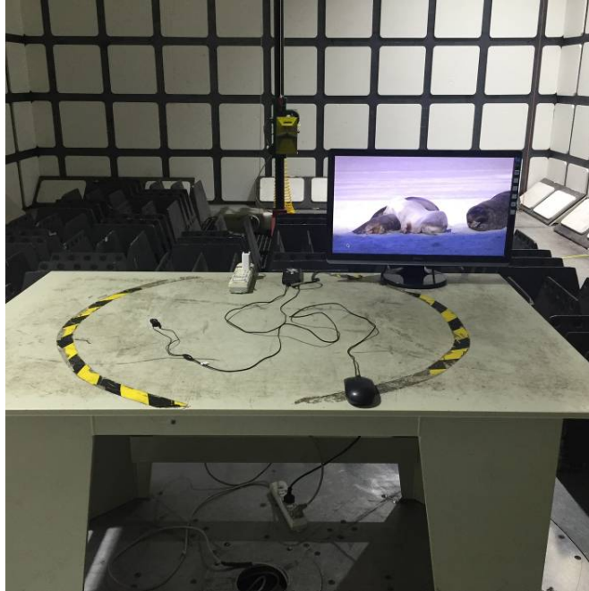
Radiated Emissions – Front View (Above 1 GHz)
