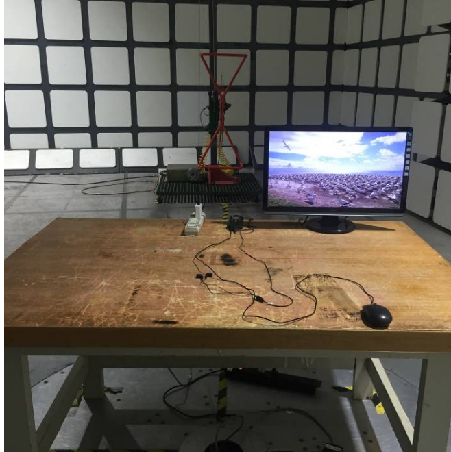
Radiated Emissions – Front View (Below 1 GHz)
