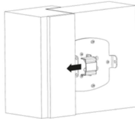
**7** Fit the Receiver on top of the Positioner.
