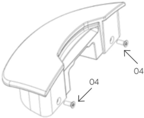
**11** Fit the lock on the base placed on the door.
