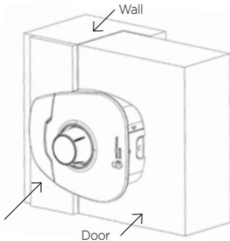
**2** Place the base of the wGravity at the desired height and flush with the edge of the door.
