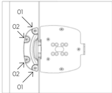
**9** Once the receiver is installed, you can remove the positioner from the base.
