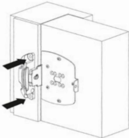
**8** Fix the receiver, together with the necessary spacers.
