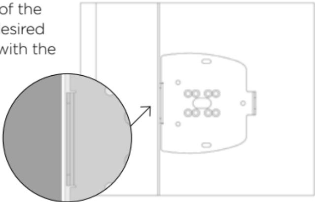
**3** Anchor the base with the wGravity with the upper and lower straight slot. *Do not squeeze too much to allow movement of the base.*
