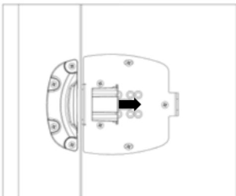
**10** Place the cover trim with its two corresponding screws.
