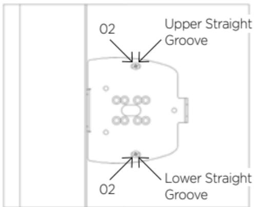
**4** Using the straight grooves finish adjusting the base to the door.
