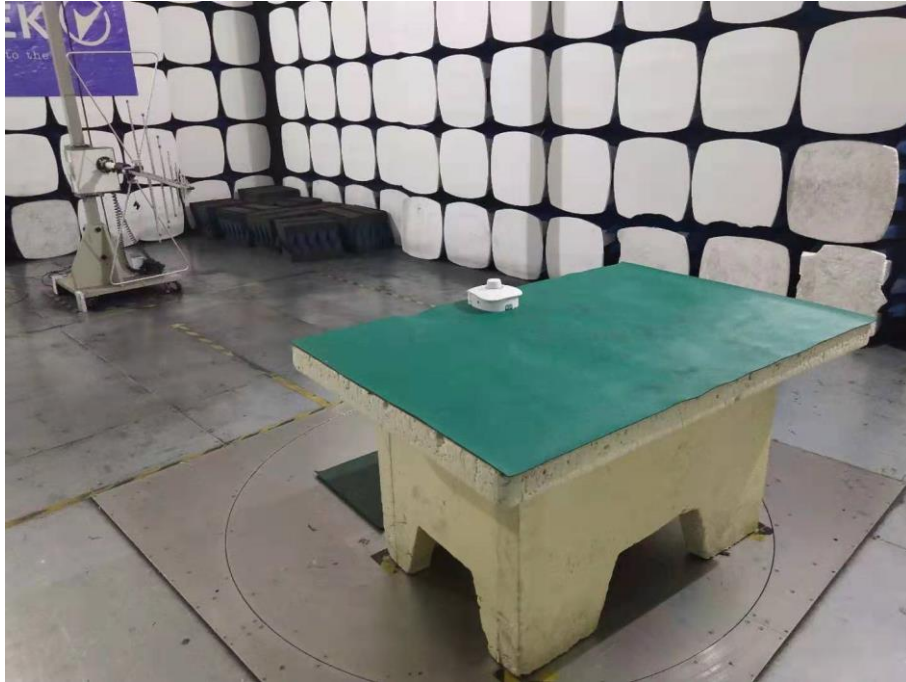
Photograph 1: Set-up for Radiated Spurious Emission, Up to 1GHz
