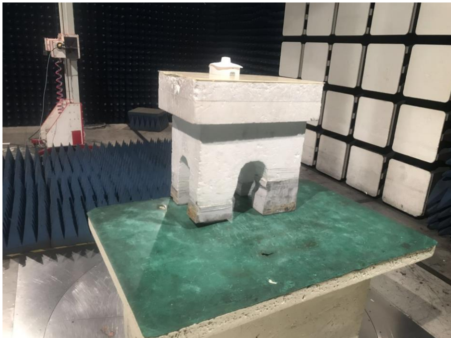
Photograph 2: Set-up for Radiated Spurious Emission, above 1GHz
