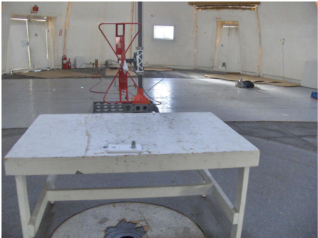
Test Set Up Photograph - Radiated - Above 1000MHz
