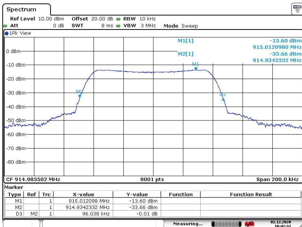
**Occupied bandwidth—power bandwidth (99%) measurement procedure**
