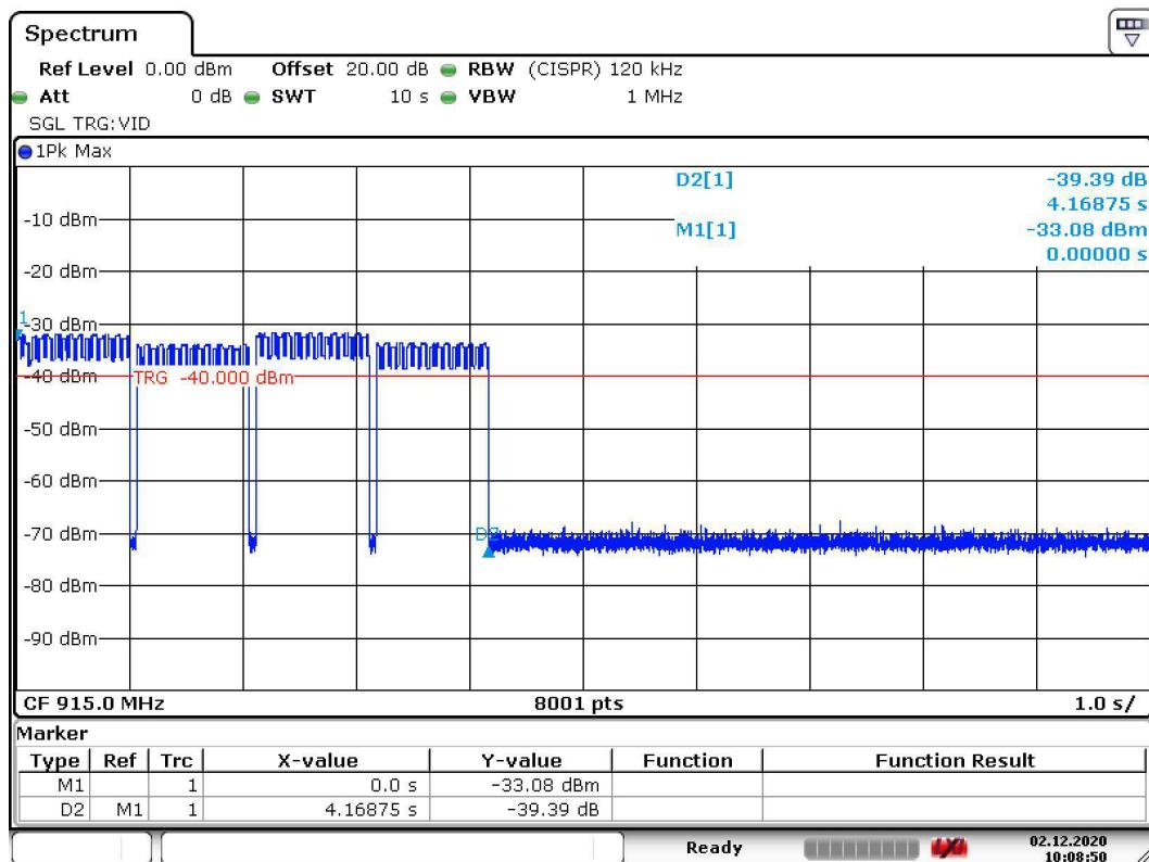
20dB bandwidth measurement procedure
