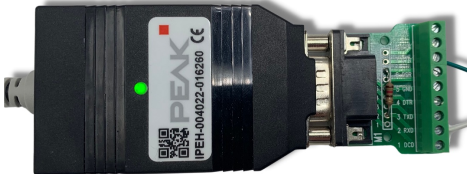
Figure 4. PEAK-CAN USB converter connected to O-79 cable (pin 2 is CAN LOW, pin 7 is CAN HIGH).
