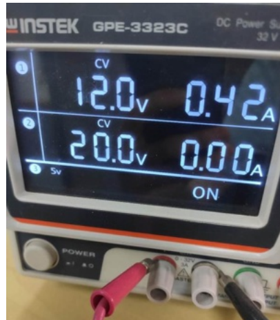
Figure 3. O-79 voltage and current draw in standby mode
