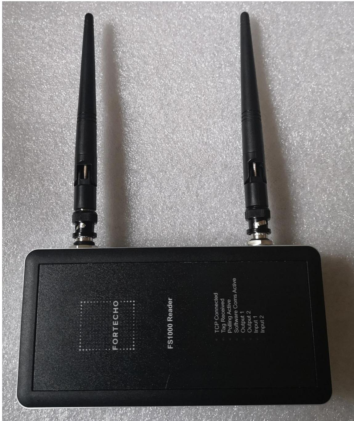
The FS1000 is shown below with a pair of FS-BNC90 antenna fitted in the right angle configuration.
