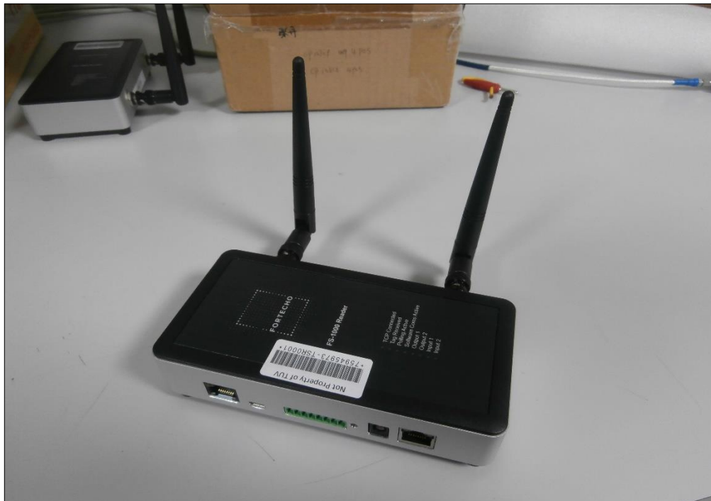
Figure 1 - Reader 433 MHz - General View
