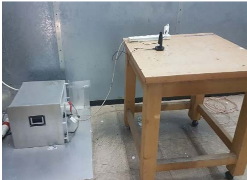
Photo 6. Conducted emissions test setup (Charging)
