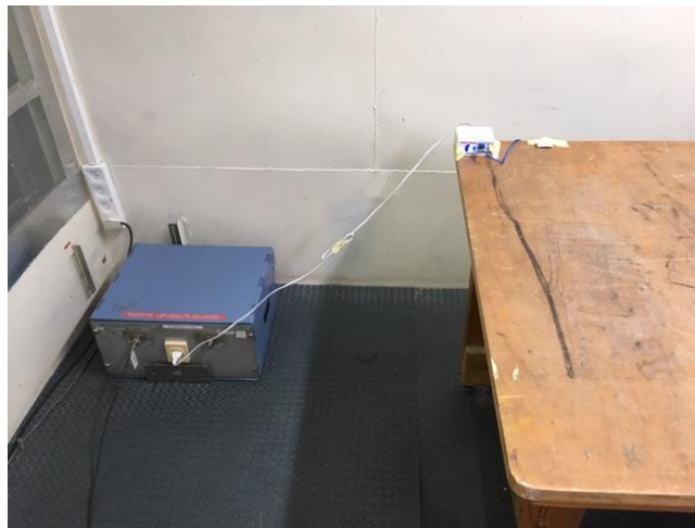
Photograph 8.1.1 Setup for conducted emission measurements
