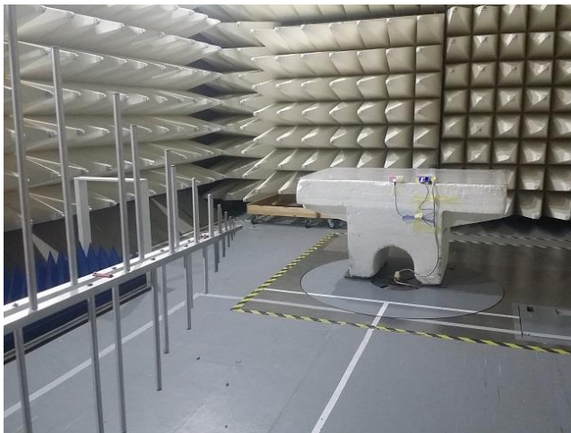
Photograph 8.2.2 Setup for radiated emission measurements, EUT cabling
