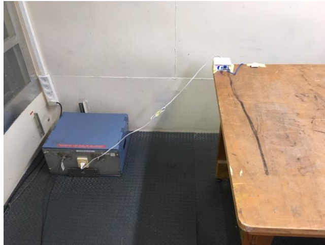
Photograph 7.6.1 Setup for conducted emission measurements
